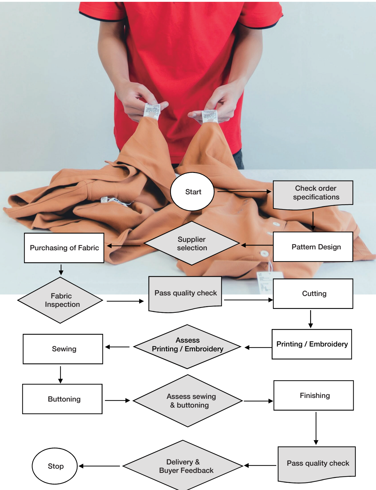
Quality Control in a Single Process Flow of Sewing Chart >> By SECXON
